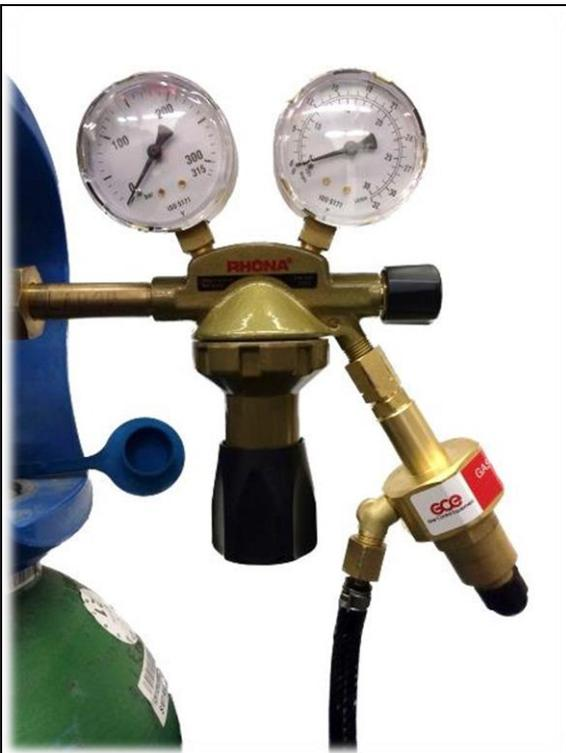
Attach gas hose from cable bundle to outlet of the shielding gas saver and reestablish gas supply to the welding system.
