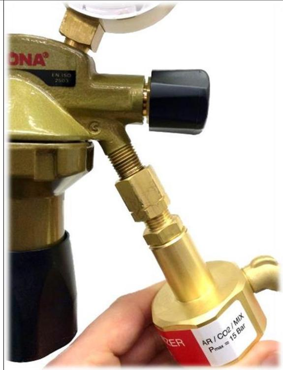
Set shielding gas saver on  $\frac{1}{4}$ " thread of the pressure regulator and tighten with jaw spanner 17mm.
